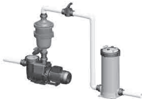
Installation with 2 way shut off valve
