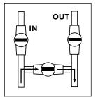
When your valves position are as shown on Figure 1, the water is bypassing the pool heat pump.
