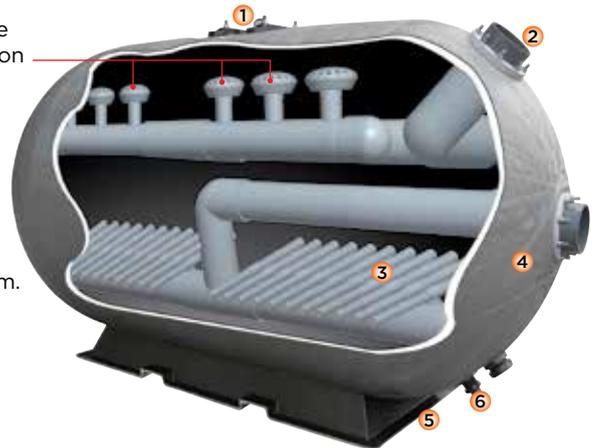
**The Micron Horizontal Filter is a space-saving high performer; its compact horizontal design allows installation with minimum waste of space. The shape of the Micron Horizontal filter is both attractive and functional. The spherical ends are designed to give uniform flow from both inlet and outlet collection assemblies. Micron Horizontal filters are available with a 500mm (M) filter media bed and a 1200mm (MD) filter media bed.**
